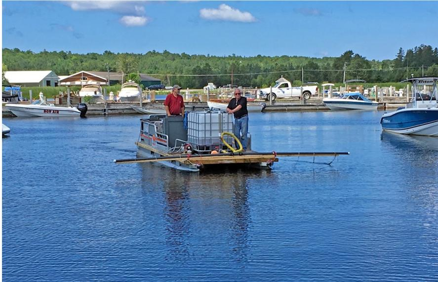
Mt aqueous suspension was applied through a manifold constructed from PVC pipe.
